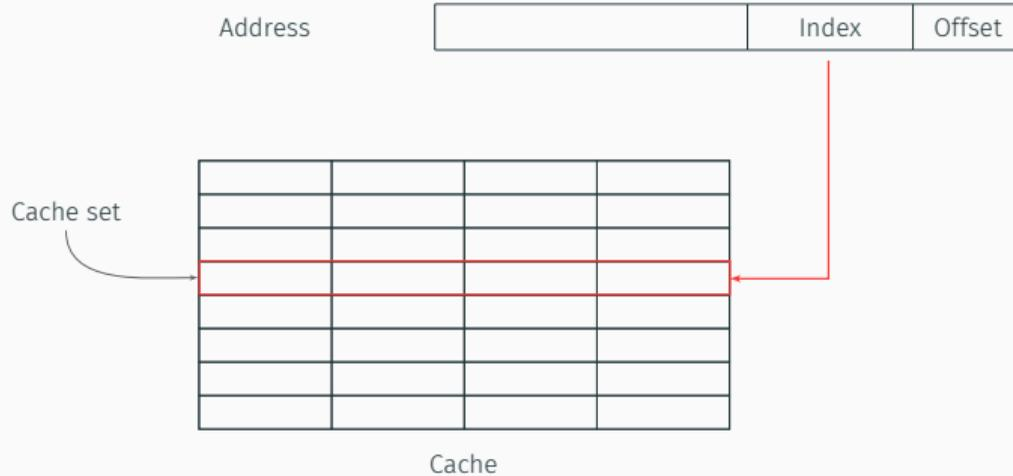
Data loaded in a specific **set** depending on its address
